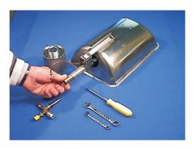
8. Locate brass venturi within the burner pipe.
