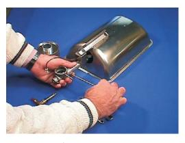
6. Loosen 2<sup>nd</sup> screw in the tee piece.
