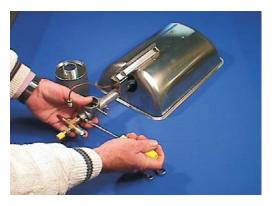
4. Loosen 1<sup>st</sup> screw in the tee-piece.
