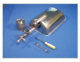
3. Rotate thermocouple out of your way.
