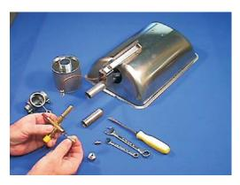
13. Remove interior coil from safety device.
