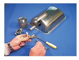
10. Grasp the safety device/jet holder assembly, taking care to not put pressure against the by-pass button. Attach your 5/16" or 8mm wrench to the hex head on the jet.
