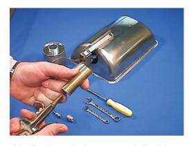
16. To clean the brass venturi, first blow out the interior with compressed air.
