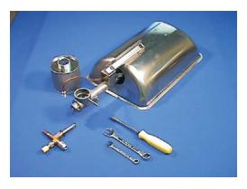
5. Remove the safety device/jet holder assembly from of the tee piece.
